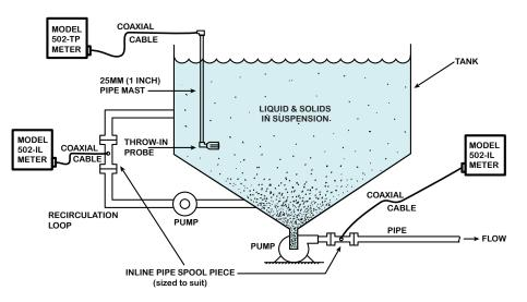
Markland's Suspended Solids Density Meter uses the attenuation of ultrasound to measure silt, sludge and slurry concentrations, and operates in the region between turbidity meters and nuclear gauges.
