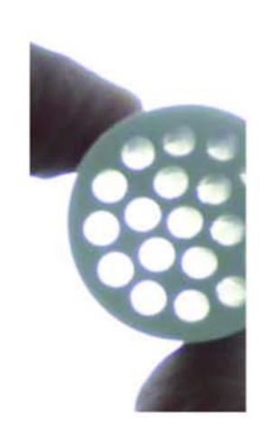
微滤/MF 孔径Pore Size: 1.2 μm, 0.5 μm, 0.2 μm, 100nm
