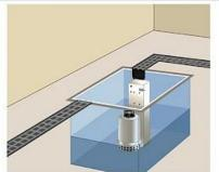
The robust insertion unit and integrated pump is located below ground level and can be installed outside within a perimeter flood defence or inside a building or property. A drainage channel or gully allows flood water to enter the sump where the insertion unit is located.
