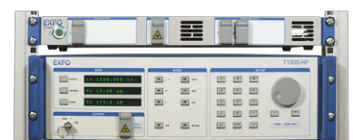
Figure 5. Rackmountable solution for both (top) CT440 and (bottom) CT440-PDL
