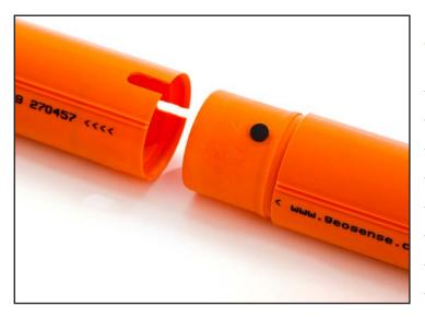
Geosense® QJ Inclinometer Casing is a quick connecting casing, precision extruded from ABS, with four precise keyways formed at 90 degrees which allow accurate installation of portable and in-place inclinometers.
