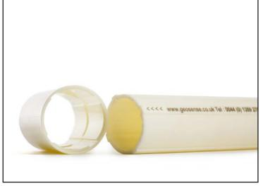
Geosense<sup>®</sup> XC (External Coupler) Inclinometer Casing is precision extruded from ABS, with four precise keyways formed at 90 degrees which allow accurate installation of portable and inplace inclinometers.
