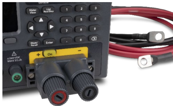
Figure 1. Detachable high current front binding post.
