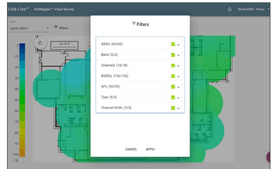
Filters allow you to choose the types of devices and network configurations to be shown.
