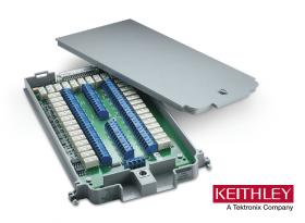
The 7708 plug-in module offers 40 channels of 2-pole or 20 channels of 4-pole multiplexer switching that can be configured as two independent banks of multiplexers. The built-in CJC sensors automatically linearize thermocouples, making the 7708 ideal for RTD, thermistor, and thermocouple temperature applications. It is also well suited for mixed-signal measurement applications that require multi-point monitoring, such as environmental stress screening.
