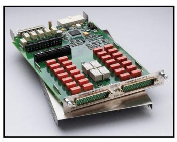
The Model 3740 offers 28 general-purpose form C channels that are ideal for routing power or other control devices. For higher power applications of up to 7A, four additional high current form A channels are provided.
