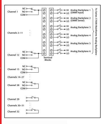
**RELAY SWITCH CONFIGURATION:** 32 general purpose independent channels. 28 channels of Form C switching at 2A and 4 channels of Form A switching at 7A. Relays can be connected to each other and backplane via removable terminal blocks.
