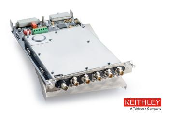
The 3765 Hall Effect Card is intended for those who want to assemble their own economical Hall test systems. It can also form the foundation of a full Hall Effect system. Used along with the free software, the Keithley Hall Effect Test Suite (KHETS), the 3765 is easily paired with Keithley DMMs, current sources, and ammeters. The card and KHETS software take advantage of the built-in DMM in the 3706A so that an external voltmeter is not required for measurements.
