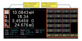
LCR-8200(A) Series allows users to select and arrange measurement parameters. Users can select at least one parameter to maximum four parameters from the 17 measurement parameters according to the measurement requirements and the presentation order can also be arranged in a desired manner. The set parameters can be stored in internal/external memory groups for subsequent recalls.
