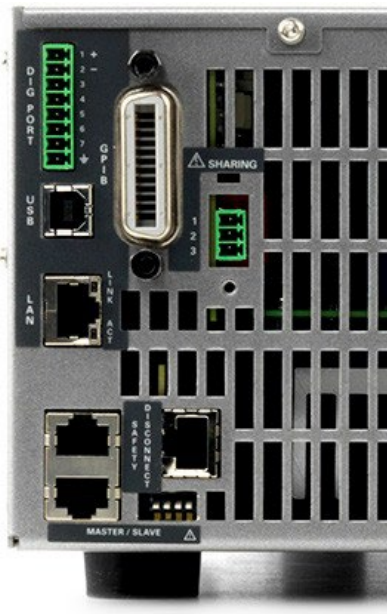
Figure 6. Digital control port on rear panel
