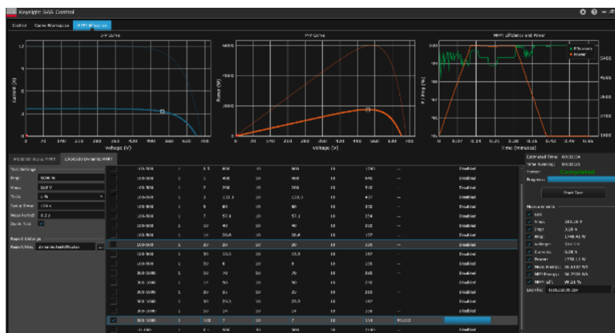
Figure 3. DG8901A dynamic EN50530 MPPT test
