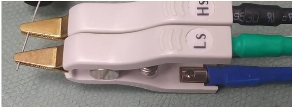
Figure 4 Use a short wire to do the short-circuit calibration
