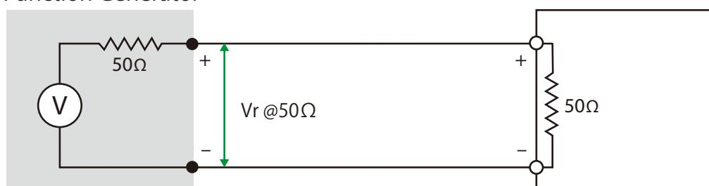
AFG series: 1 mV<sub>pp</sub> to 10 V<sub>pp</sub> (into 50Ω)
