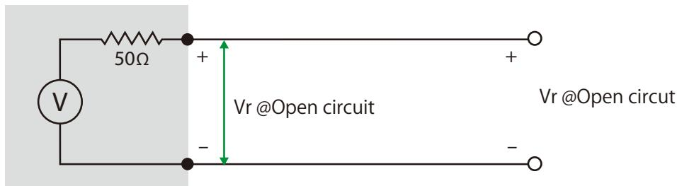
$V_r @ 50\Omega \times 2 = V_r @ Open Circuit$
