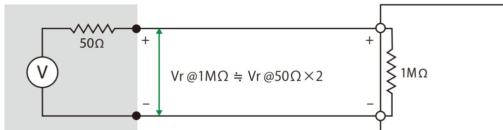
AFG series: 2 mV<sub>pp</sub> to 20 V<sub>pp</sub> (@1MΩ)
