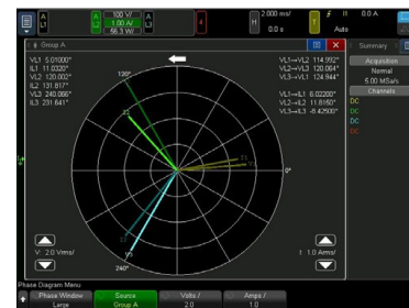
Figure 4. Phasor diagram for phase relationship analysis
