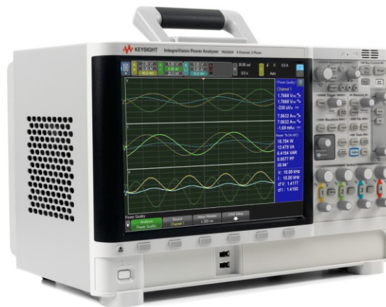
Figure 1. PA2203A IntegraVision Power Analyzer 4 Power Channels, 3-Phase Analysis
