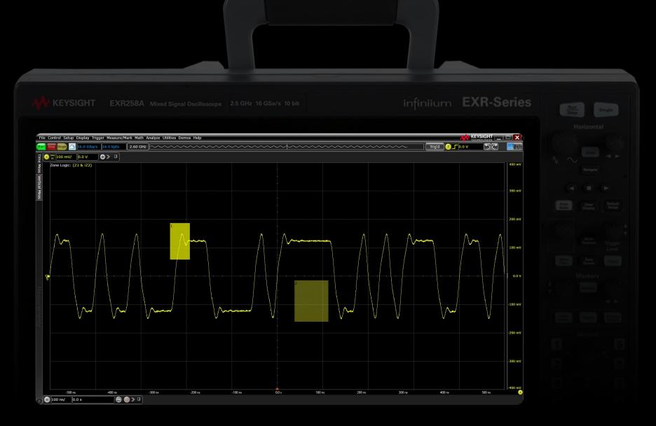
D9110SCNA InfiniiScan using the Zone trigger mode to isolate a specific waveform
