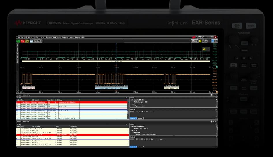
D9110AUTP Automotive decode/trigger letting a user set up a CAN and LIN decode simultaneously to look at a serial bus gateway
