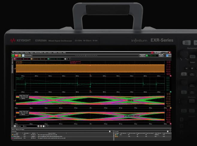
D9110POWA Power Integrity application showing the user effects of power supply induced jitter in their design
