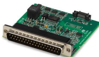
TS-15110 Analog Output Module 10 V, 16 bit, 4 ch
