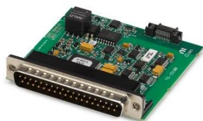
TS-15100 Analog Input Module 250 kS/s, 16 bit, 32 ch
