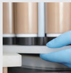
Rotor raised when safety door is opened to a \geq 90^\circ
