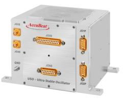
probe Jupiter's atmosphere by following the phase variations of the radio waves passing through the atmosphere while the spacecraft transmits to earth using AccuBeat's ultra-high stability frequency source.
