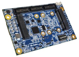
Astro makes use of a high density, board-to-board connector that allows for use with break-out boards.
