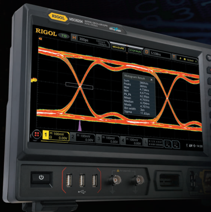
Perform eye measurement on the 622 Mb/s signal.
