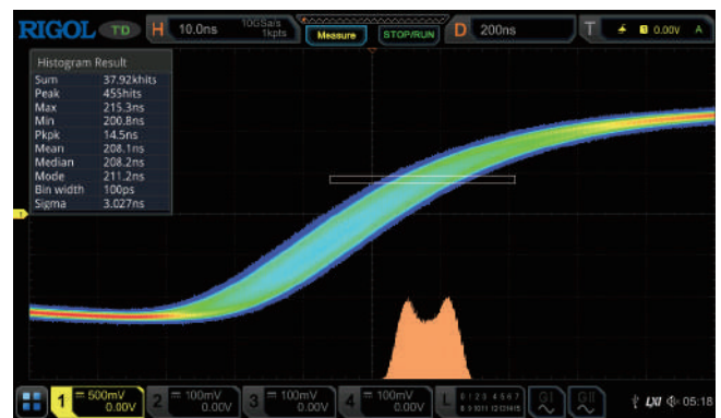
Histogram of Horizontal Waveforms
