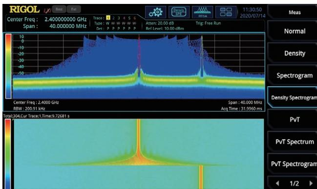
Density spectrum for you to visualize how frequently signals occur
