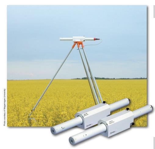
The Scintec SLS20 Scintillometer measures turbulence, heat flux and momentum flux by purely optical means. In combination with other meteorological sensors the system can determine latent heat flux or evaporation.
