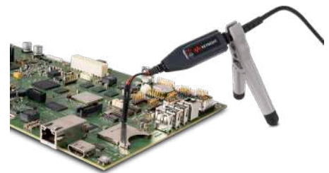
DP001xA Series probe using socketed Y-lead
