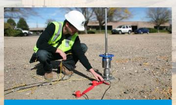
Two additional radial geophones allow for two layer analysis by AASHTO Odemark Method of Equivalent Thicknesses approach
