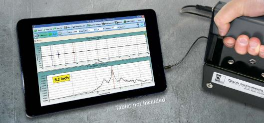
**Detects: Honeycomb, Voids, Cracks and Delamination**
