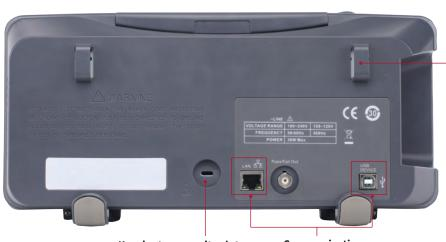
Kensington security slot Helps to secure your oscilloscope and prevent theft.
