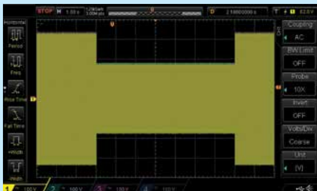
Three Phase Voltage Drop Test Captured
