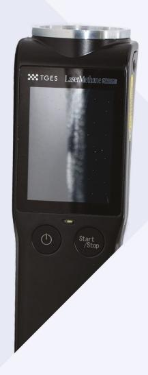
The detector measures the characteristics of methane, which is absorbed into the laser beam (infrared beams) of a specific wavelength (infrared absorption technology). The directed laser reflects back a diffused beam from the target, where the device will receive the reflected beam and measure the absorptivity of the beam, that is then calculated into methane column density (ppm-m).
