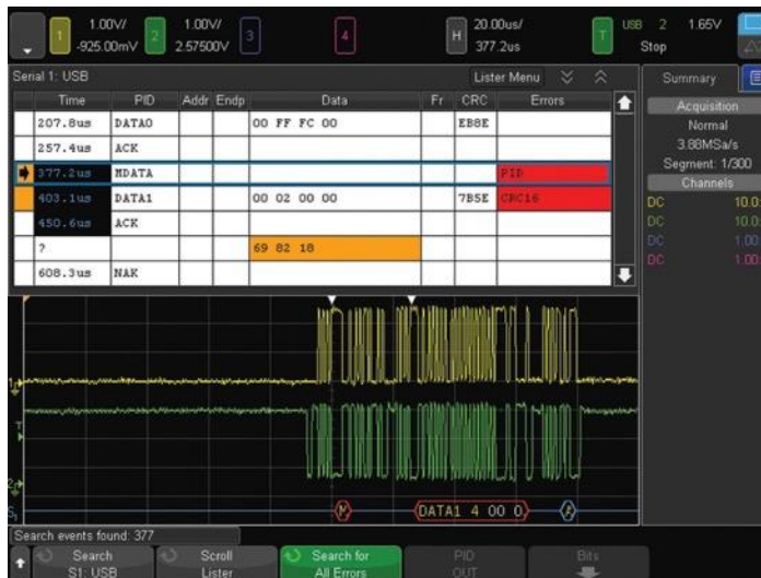
Figure 21. USB 2.0 trigger, decode and "lister" display.
