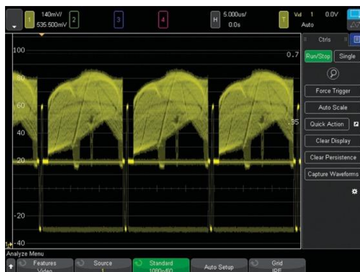
Figure 27. Triggering on 1080p HDTV signal analysis.
