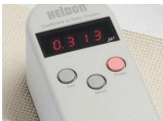
The friction meter stores several measured values in its memory and displays the measurement count and average static friction coefficient. The measurement starts by simply placing it on an object to be tested and pressing a switch, eliminating variations of result depending on the operator. Powered by AA size battery cells, the tester makes an measurement quickly and anywhere.
