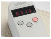
The friction meter stores several measured values in its memory and displays the measurement count and average static friction coefficient. The measurement starts by simply placing it on an object to be tested and pressing a switch, eliminating variations of result depending on the operator. Powered by AA size battery cells, the tester makes an measurement quickly and anywhere.
