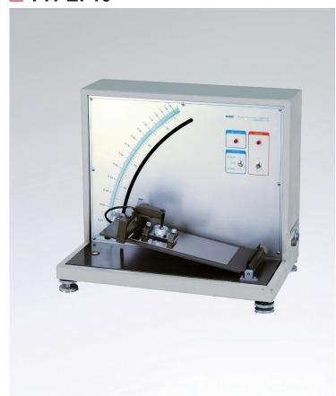
The test sample is installed on the ascending board and flat indenter. The board is equipped with a sensor that monitors the movement of the flat indenter. The ascending board at the horizontal position starts to increasingly tilt when the measurement begins. The sensor detects the motion when the flat indenter begins to slide, and stops the board
