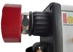
The miRoGun4.0 unit can be operated as well as a desktop instrument. Thus small particles less than 1 mm can be placed easily in the center of the measuring head being in the optical focus.
