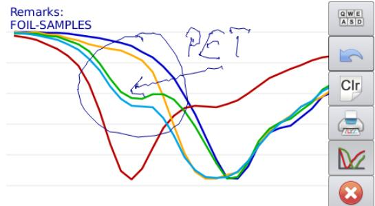
For plastic identification the unit is pressed on the surface of the sample and is measured by pressing the trigger button. Single measurements can be made as well as online (circular) measurements with a fixed trigger key.
