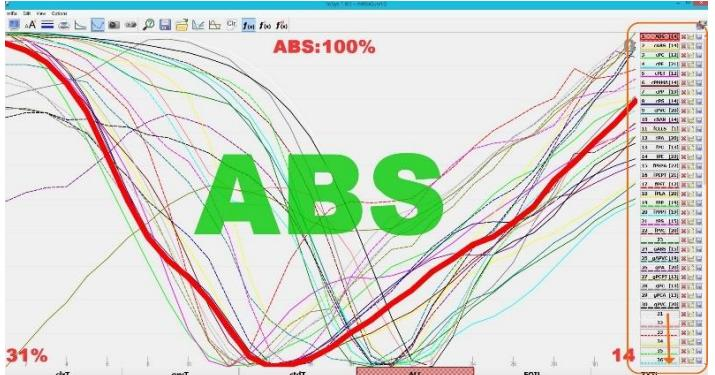
The external software enables the transmission and display of the data on the PC via USB or Wi-Fi. It allows the analysis, comparison and storage of all measured spectra on the PC, also individual printouts of the measuring report with comments. In the Analyse-mode up to 80 different spectra can be displayed at once in different colors!
