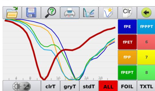
The unique way of displaying the transformed NIR-spectra on the color LCD-touch-screen allows easy look and control of the results and the comparison with other polymer, carpet/textile materials.
