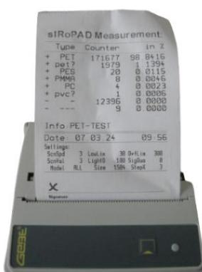
**Measurement results can be grouped, listed, arranged and printed out on the mini-plotter and/or at the connected PC-printer as an analysis report.**
