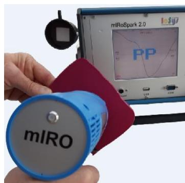
all common types of plastics, regardless of color, size, structure like films, foils, granules, solid, carpets and textiles can be identified with additive elements like fire retardants and heavy metals.
