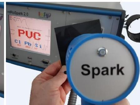
to the sample surface. The analysis begins by pressing the start trigger of the pistol grip. After one second an integrated color TFT-screen displays the recognized polymer. The measuring pistols each are connected to the instrument with a 2 m cable and protective hose. The optical signals are transported via fiber cable to the spectrometer systems. Parameter settings as well as control can be effected by an integrated touchscreen.
