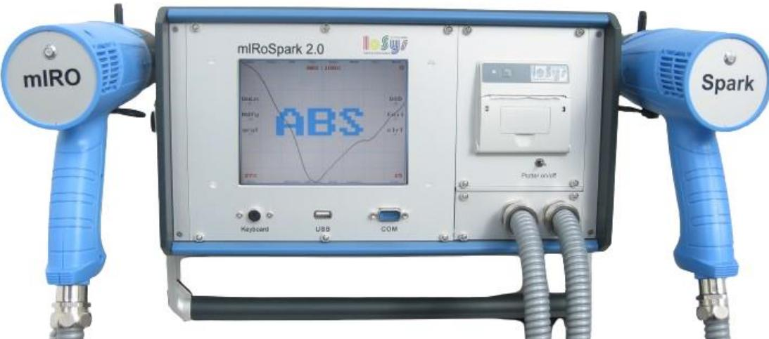
characteristic absorption behaviors of different polymer types are used in that spectral region. The polymer sample is radiated with an NIR-light and the reflected light of the measuring place is analyzed using a near infrared detector array.
