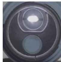
surface using a train or defined high-current sliding sparks between the electrode gap within ~1sec. The polymer- and additive-components in the spark plasma are vaporized, atomized, ionized and activated to emit spectral characteristic VIS/UV-light radiations.
