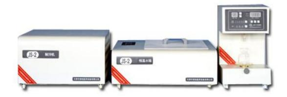
JS-2 Gelatin gel strength systems is the latest development production of our company, which is the requisite instrument in detecting jelly strength of gelatin. The instrument design and technical specifications of this tester reached or surpassed the advanced level of this kind of instrument in the world.
