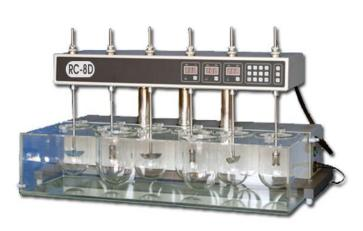
RC-6/8 Series Dissolution Testers are the latest development and production of our company, which is the requisite instrument in detecting dissolution of tablets, capsule etc. The design and technical specifications of these testers reached or surpassed the advanced level of this kind of instrument in the world. All of our lab instruments are designed and manufactured in according to USP Specifications.
