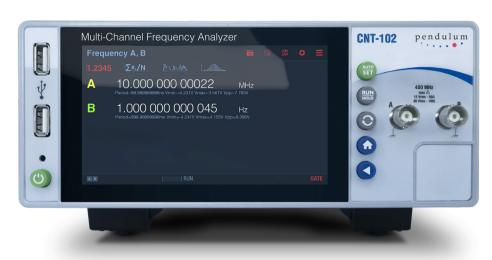
The Pendulum CNT-102 is a *new* affordable model in the CNT-100 family for superperformance *multi-channel* frequency and time-interval analysis in a bench-top unit. You can track parallel frequency, phase or time simultaneously on 2 input channels on the large graphic screen. These instruments feature gap-free measurements, and have 14 ps time resolution, up to 13 digits/s frequency resolution, and a measuring speed of 1M results/s.
