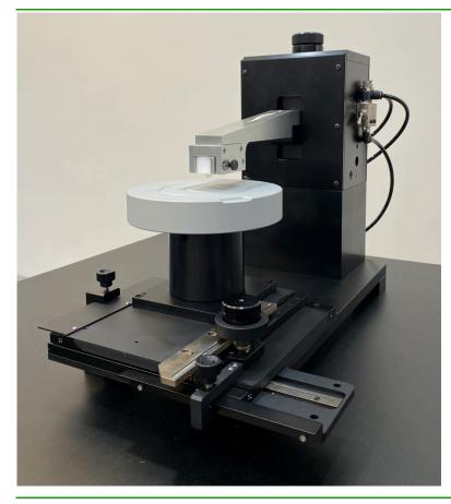
SR-4 equipped with chuck stage and hot chuck
