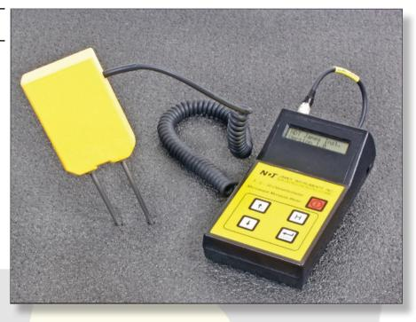
times greater than most aggregates andcements, changes in water content directly effect the sensor output. An average of five to ten readings is normally taken in order to ensure a valid reading. This output is then converted by the integrated microprocessor and moisture content is displayed directly.
