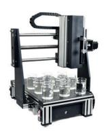
MULTI VESSEL DIP COATING SYSTEM
