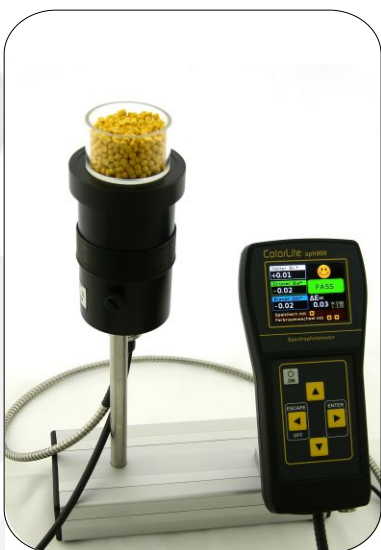
MA38 Set for measuring samples with the ColorLite sph900
