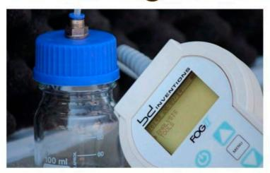
On the go determination of the total inorganic carbon as equivalent calcium carbonate content with **GPS** technology
