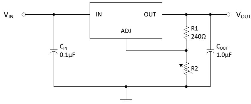
$$V_{OUT} = V_{REF} (1 + R2 / R1) + (I_{ADJ} \times R2)$$
