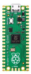
Raspberry Pi Pico is the debut microcontroller-class board from Raspberry Pi. Built around our RP2040 silicon platform, Pico brings our signature values of high performance, low cost, and ease of use to the microcontroller space.
