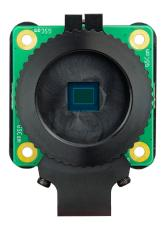
The Raspberry Pi Global Shutter Camera is a specialised 1.6-megapixel camera from Raspberry Pi that is able to capture rapid motion without introducing artefacts typical of rolling shutter cameras. It is ideally suited to fast motion photography and to machine vision applications, where even small amounts of distortion can seriously degrade inference performance.
